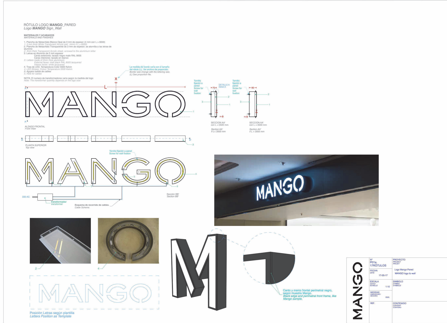
EQ-30b Signage Detail (Filed Under Separate Permit)
